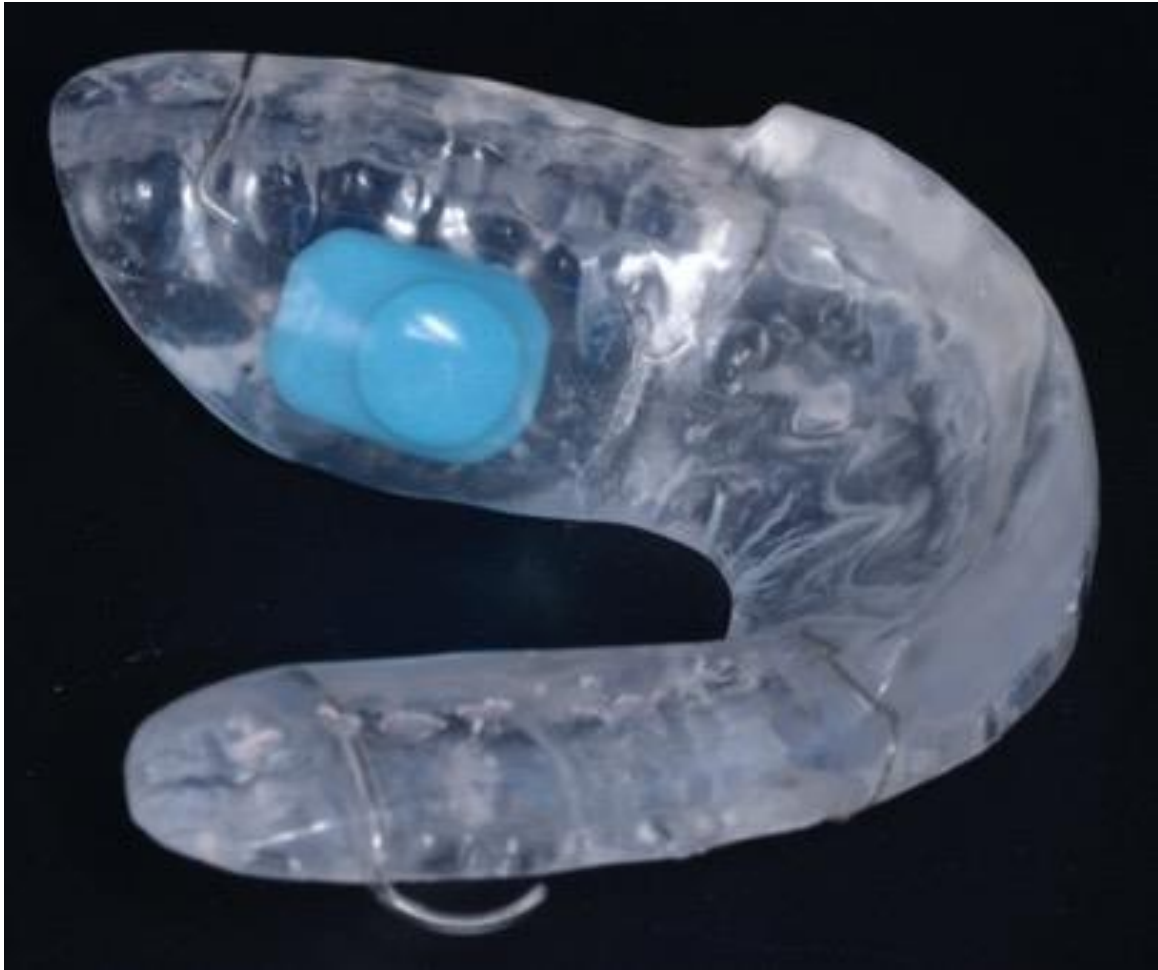
Figure 2.8. Maxillary occlusal device with incorporated microsensor embedded during processing.
