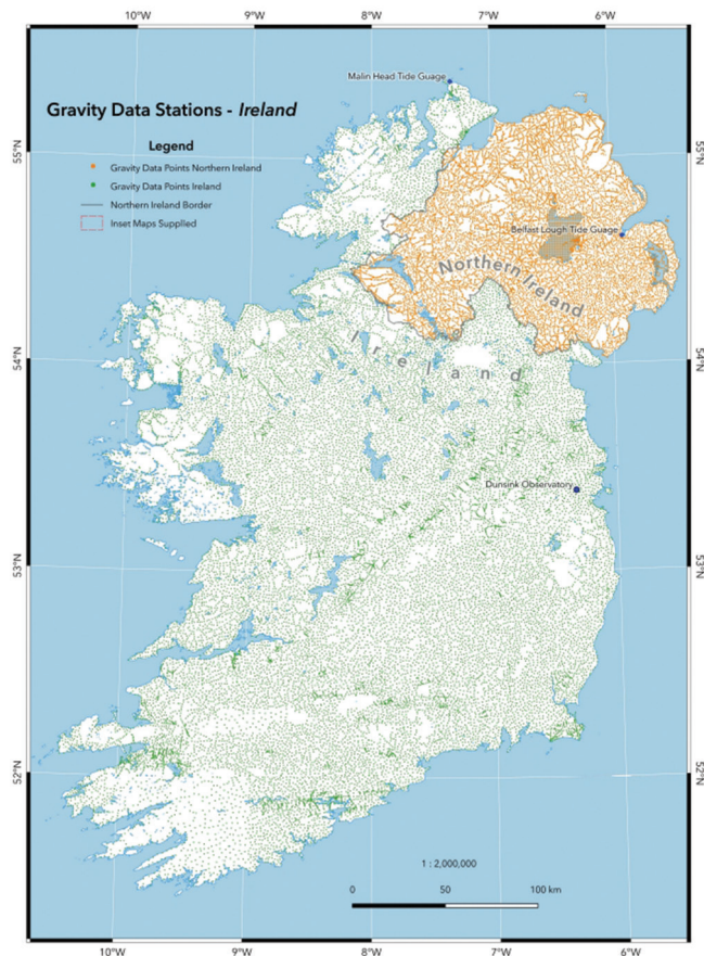
Figure 1. Distribution of gravity data in Ireland . Each data point represents a measurement collected by the DIAS (23,285 data points) and GSNI (11,256 data points).
