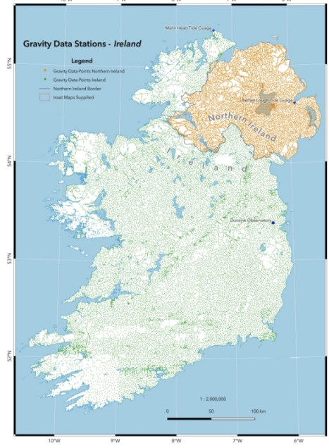
Figure 2: Distribution of gravity data in Ireland; each data point represents a measurement collected by the DIAS (23285 data points) and GSNI (11256 data points) in geodetic coordinate system.
