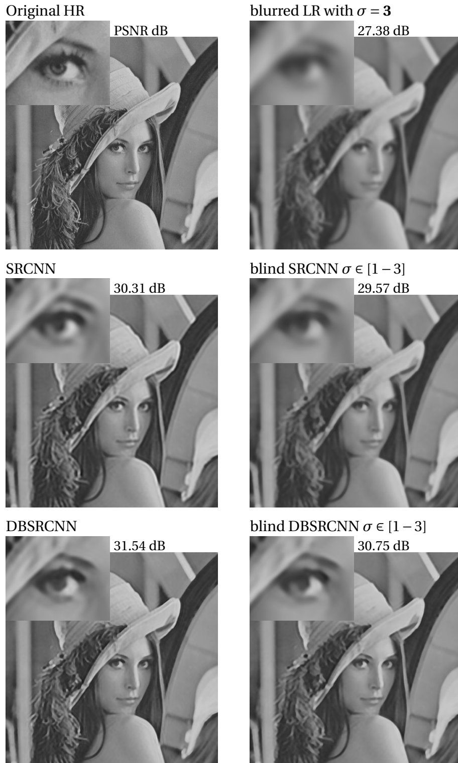
Fig. B.5 SR with SRCNN and DBSRCNN on grey-scale images after Gaussian blur with \sigma = 3 . The second and third rows show the results of SRCNN and DBSRCNN, respectively; according to the two different scenarios (the non-blind and blind \sigma \in [1 - 3] SR scenarios). Each result is accompanied by zoom and PSNR dB.
