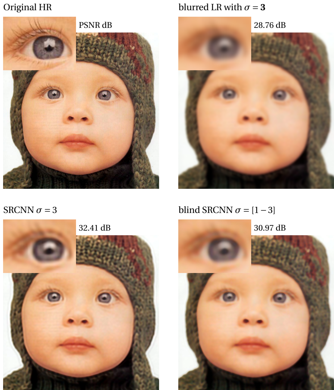
Fig. 4.3 SR with SRCNN on a colour image after Gaussian blur with \sigma = 3 . The second row shows the results of the non-blind scenario and the blind scenario. Each result is accompanied by zoom and PSNR dB.
