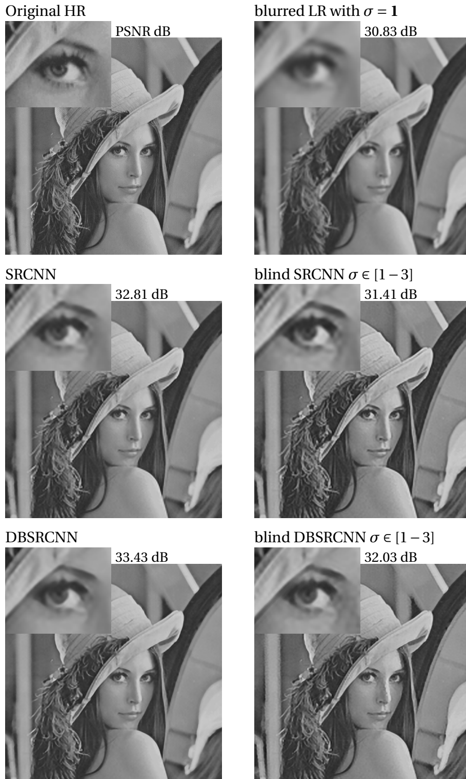
Fig. B.4 SR with SRCNN and DBSRCNN on grey-scale images after Gaussian blur with \sigma = 1 . The second and third rows show the results of SRCNN and DBSRCNN, respectively; according to the two different scenarios (the non-blind and blind \sigma \in [1 - 3] SR scenarios). Each result is accompanied by zoom and PSNR dB.
