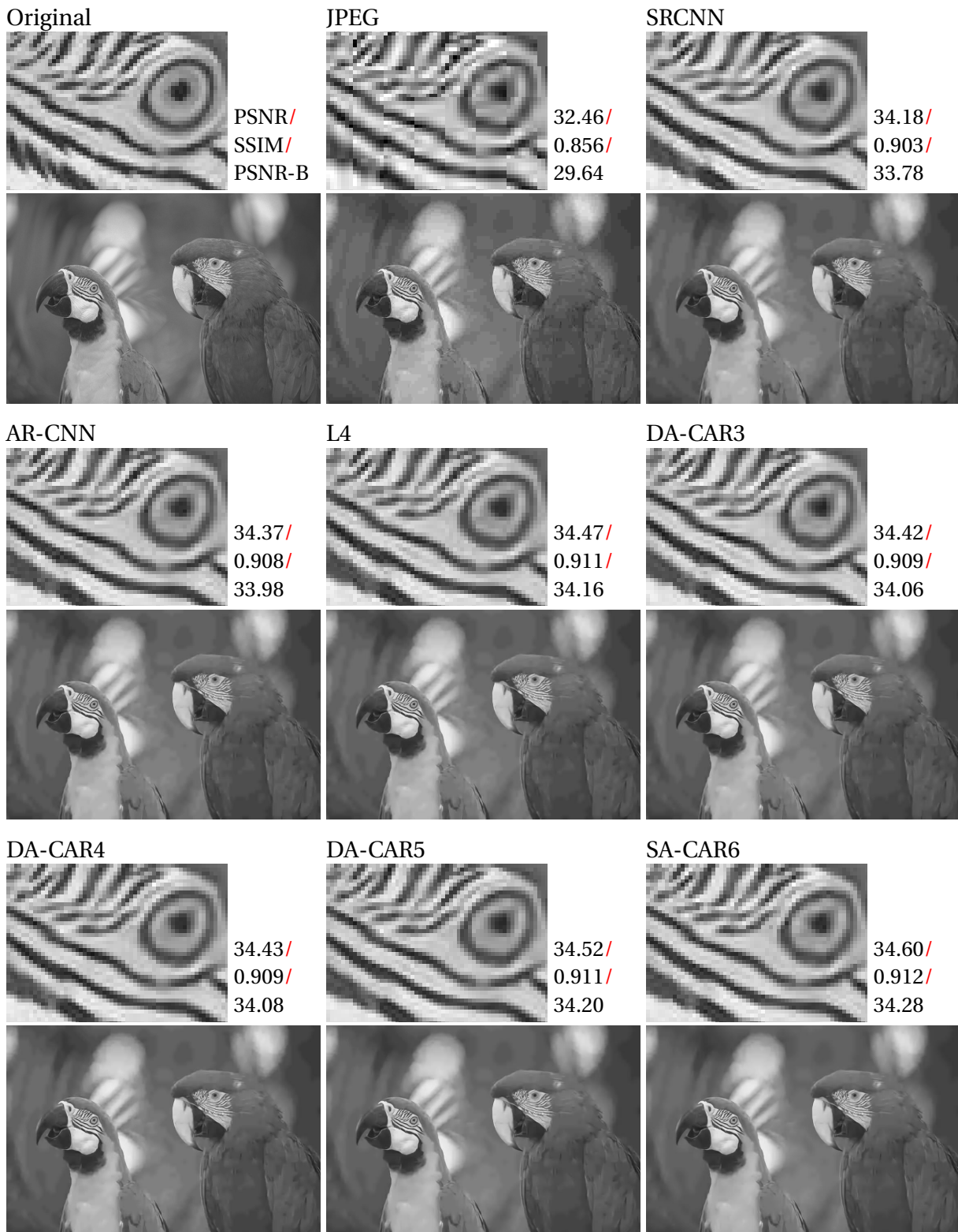
Fig. 5.4 Qualitative evaluation of reconstruction quality for parrots image using different networks for JPEG quality q = 10 . Each result is accompanied by zoom and PSNR dB/ SSIM/ PSNR-B dB.
