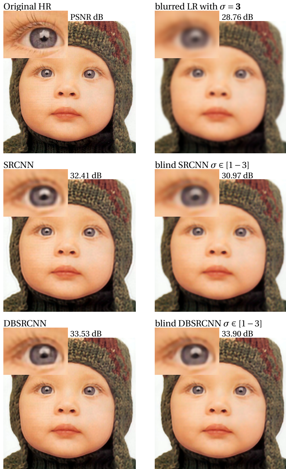
Fig. B.9 SR with SRCNN and DBSRCNN on a colour image after Gaussian blur with \sigma = 3 . The second and third rows show the results of SRCNN and DBSRCNN, respectively; according to the two different scenarios (the non-blind and blind \sigma \in [1 - 3] SR scenarios). Each result is accompanied by zoom and PSNR dB.
