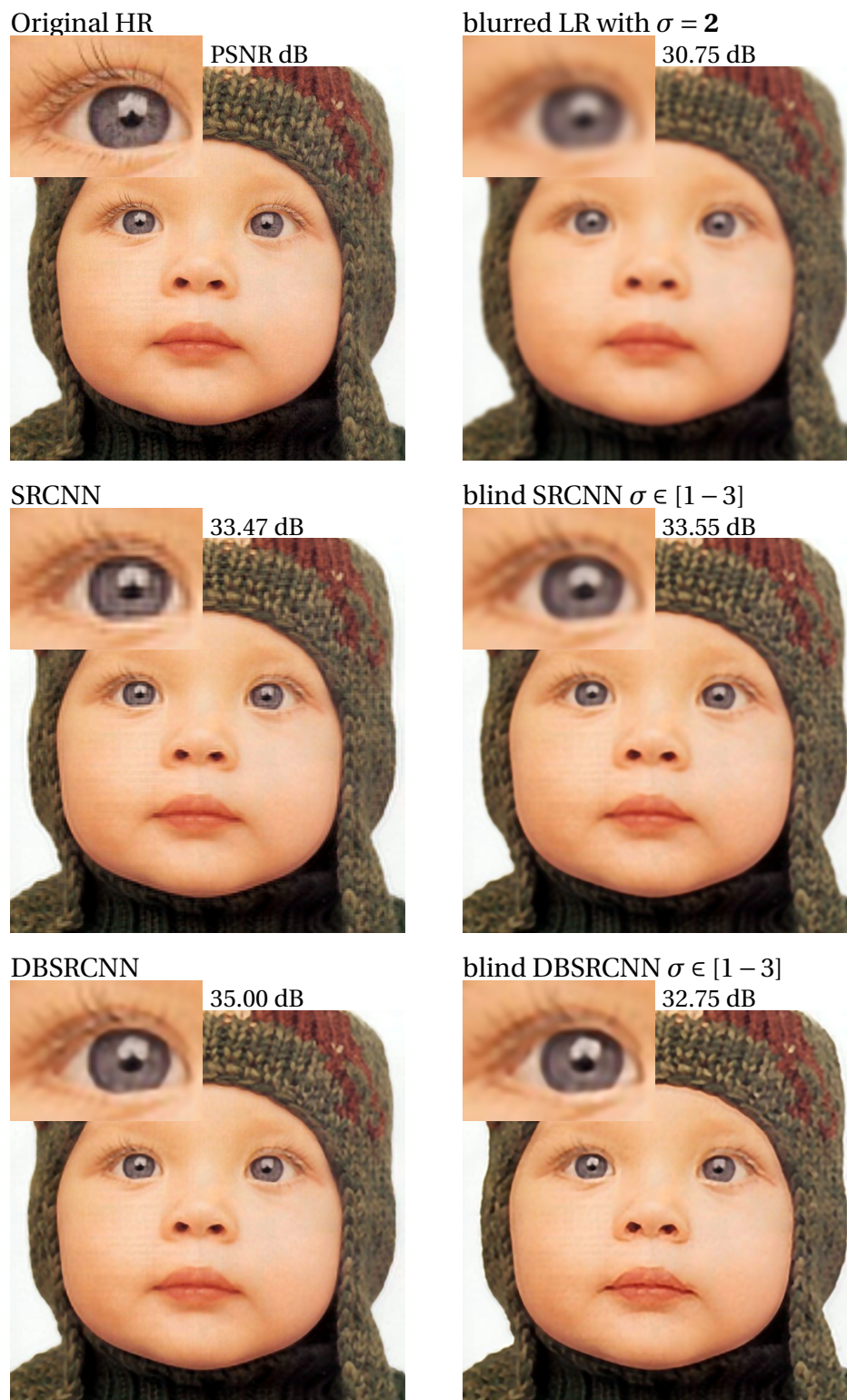
Fig. B.8 SR with SRCNN and DBSRCNN on a colour image after Gaussian blur with \sigma = 2 . The second and third rows show the results of SRCNN and DBSRCNN, respectively; according to the two different scenarios (the non-blind and blind \sigma \in [1 - 3] SR scenarios). Each result is accompanied by zoom and PSNR dB.
