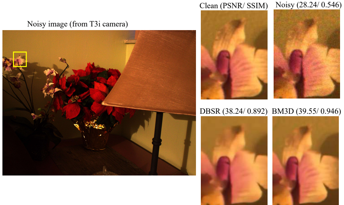
Fig. 6.3 Results of DBSR and BM3D methods on the RENOIR dataset with zoomed crops.
