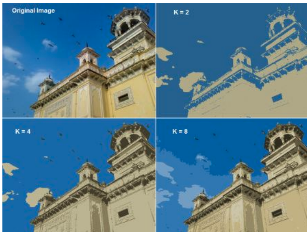
Figure 3.9: An example of reducing the colour space of an image with clustering using different cluster sizes (K) 5
