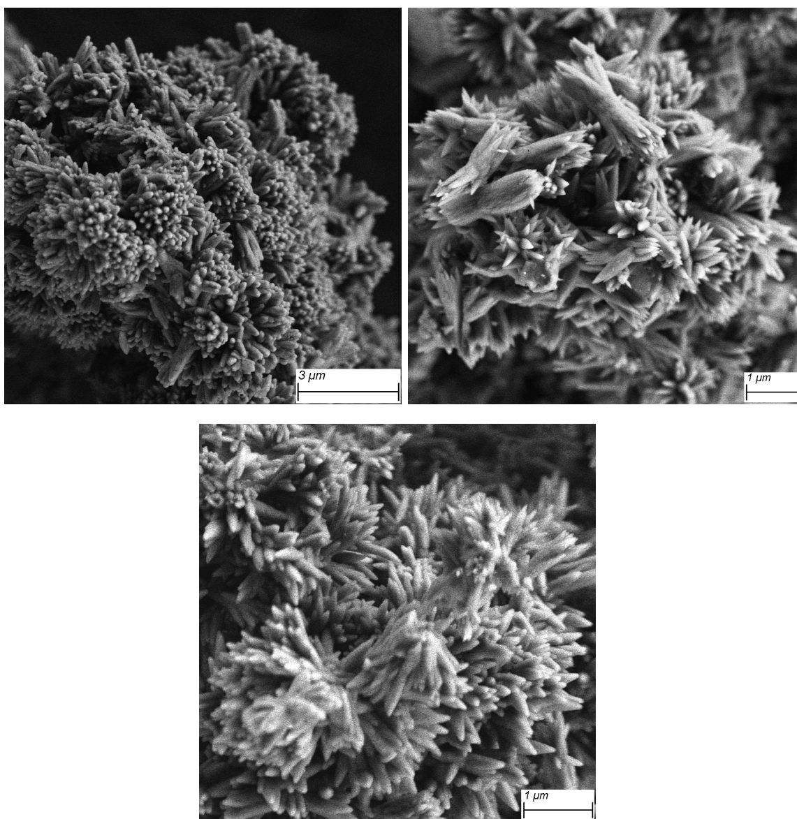
Figure 7.13: SEM images of calcite synthesised at 0.5 \text{ mol L}^{-1} \text{ Ca(OH)}_2 with \text{CO}_2 flow rates of (a) 0.3 \text{ min}^{-1} (b) 0.4 \text{ min}^{-1} and (c) 0.5 \text{ min}^{-1}
