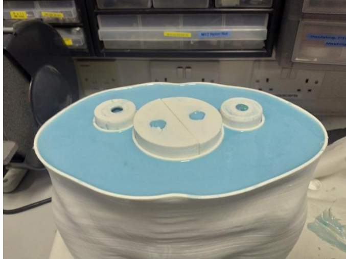
Figure 2.4. Phantom illustrating prostate and femoral heads inserts.
