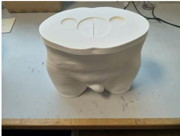
Figure 2.5. Completed 3D printed phantom
