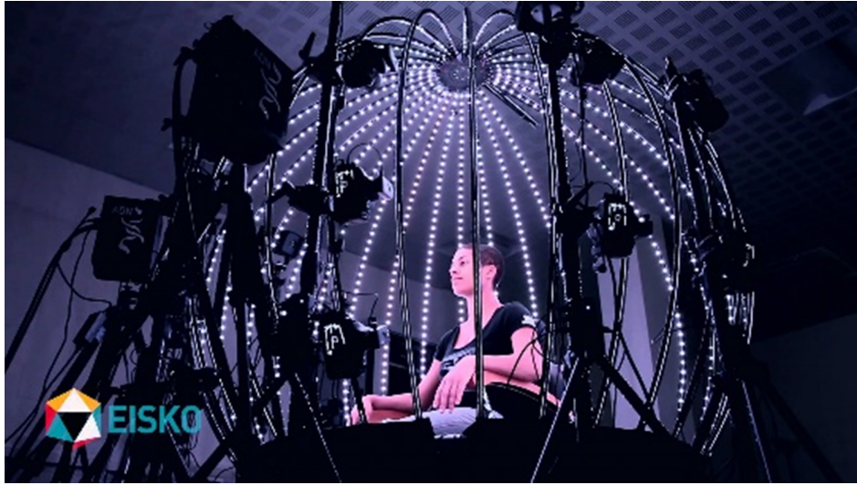
Figure 2.2: An actor being scanned in a light stage.
