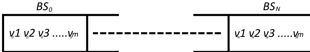
Figure 4.3: The blendshapes are serialised and stacked together in the 1-dimensional Texture Buffer Object.
