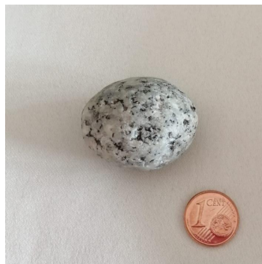
Figure 1: Hand sample of light grey equigranular phaneritic granite, with visible quartz, feldspar, biotite, and muscovite.
