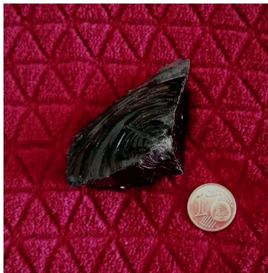
Figure 3: Hand sample of black obsidian, exhibiting concentric conchoidal fracture
