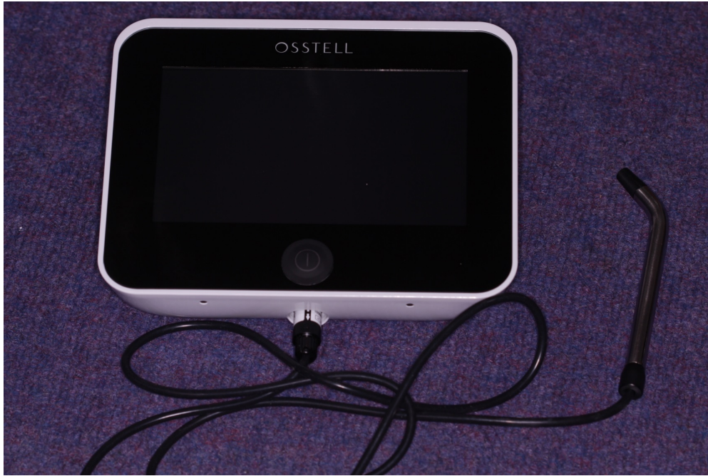
Fig 1.3 Photograph of Osstell® Mentor (Integration Diagnostics AB, Gothenburg, Sweden).
