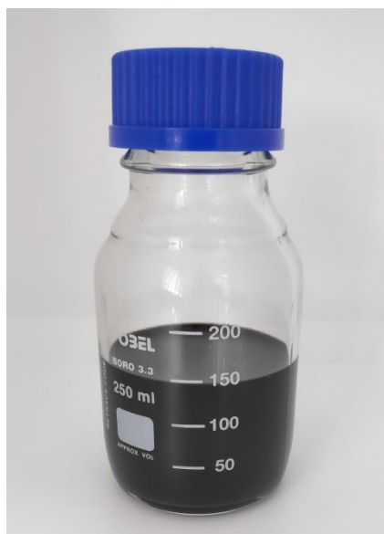
Figure S1. Digital photograph of a bottle containing an aqueous anodic graphene dispersion at a concentration of 2 \text{ mg mL}^{-1} derived from derived from 0.1 M AMP.
