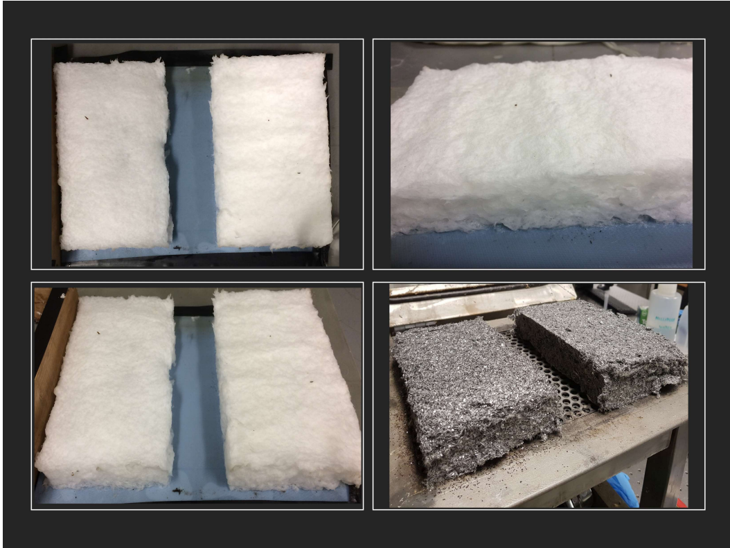
Fig 3.5: Samples left to dry on the bench in our laboratory. All samples contained Kraft fibres. The samples on the bottom right contained graphene flakes as well as Kraft fibres.
