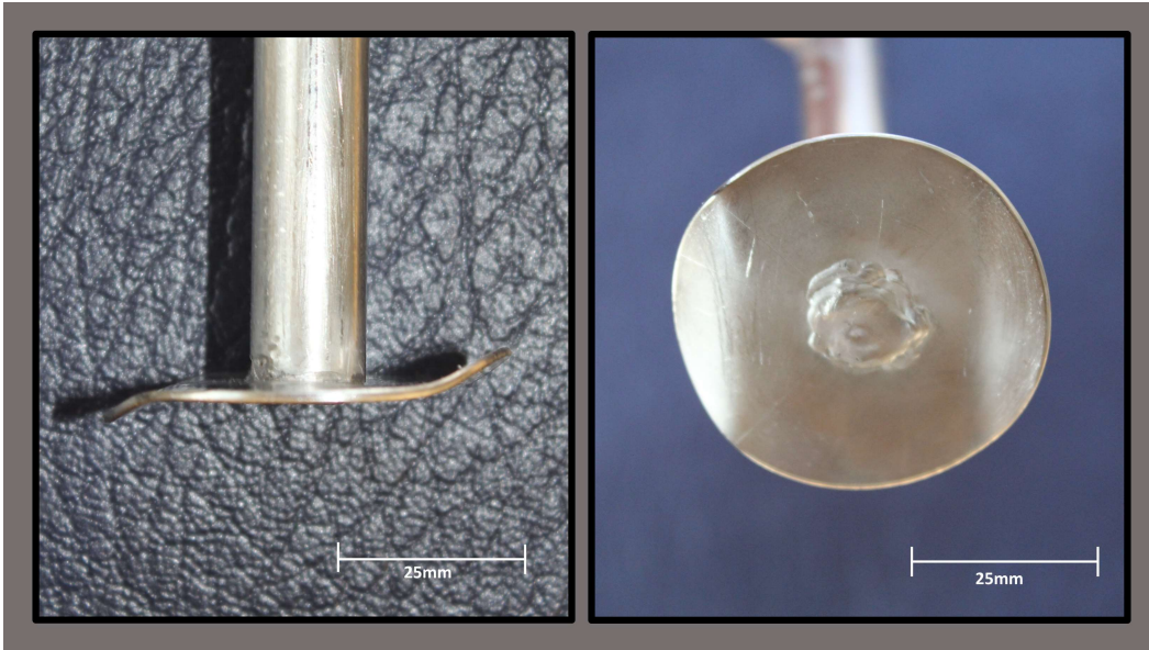
Fig 2.1: The mixing disk used to produce the aqueous foams discussed in this thesis. The image on the left shows the disk's two opposing 25^\circ bends, which entrains air into the aqueous solution by creating a turbulent flow thus producing foam of highly polydisperse bubbles. The image on the right shows a view of the disk from the underside.
