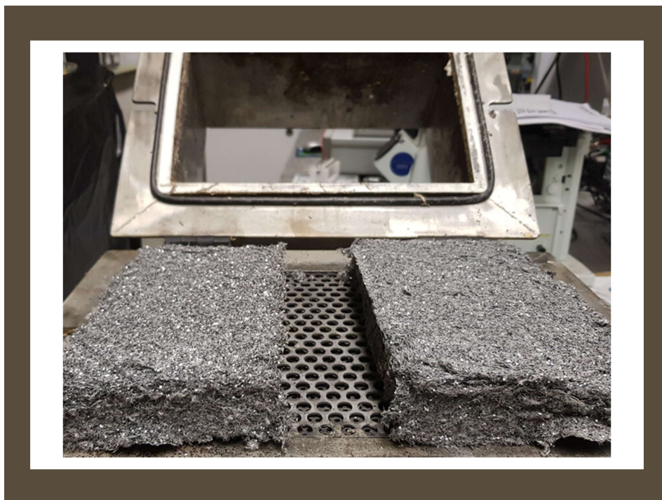
Fig 8.4: Two samples made by foam-forming. Both contained a quantity of graphene flakes and Kraft fibres. The samples were made to determine if the higher density graphene would sediment from the dispersions. No sedimentation occurred.
