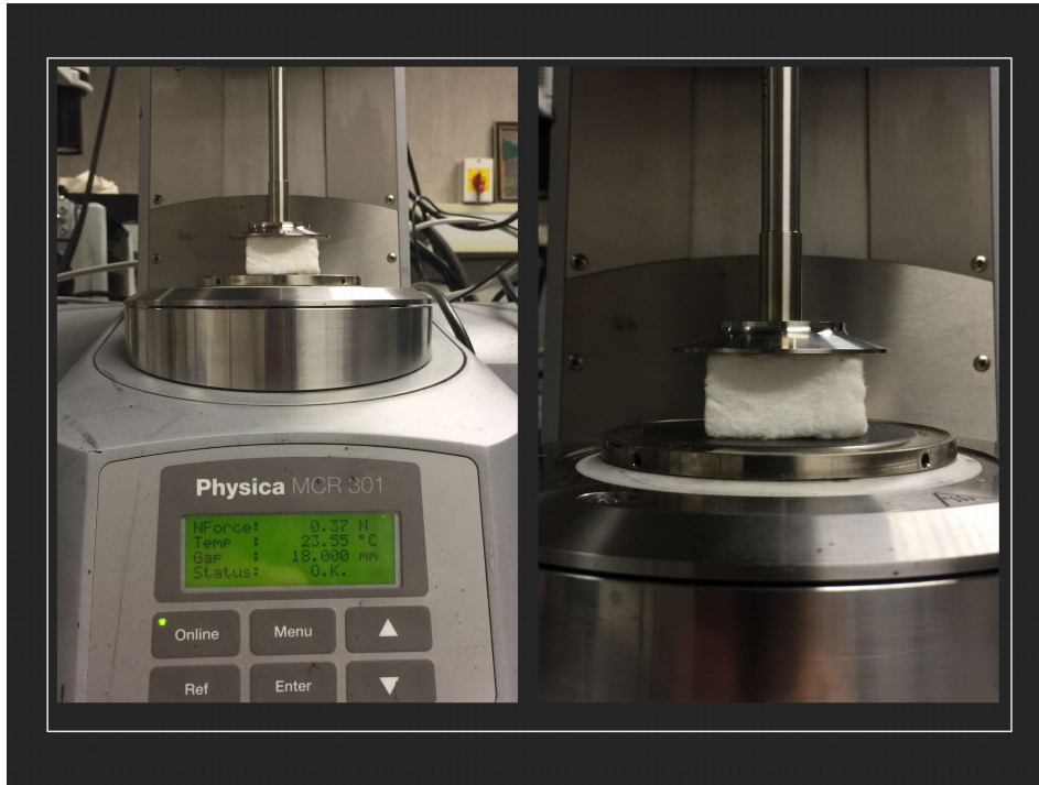
Fig 5.3: On the left is an image of the rheometer (Anton Paar Physica MCR301) used to measure the compressive response of the samples. The image on the right is a close up of one of the samples placed between the two plates of the rheometer.
