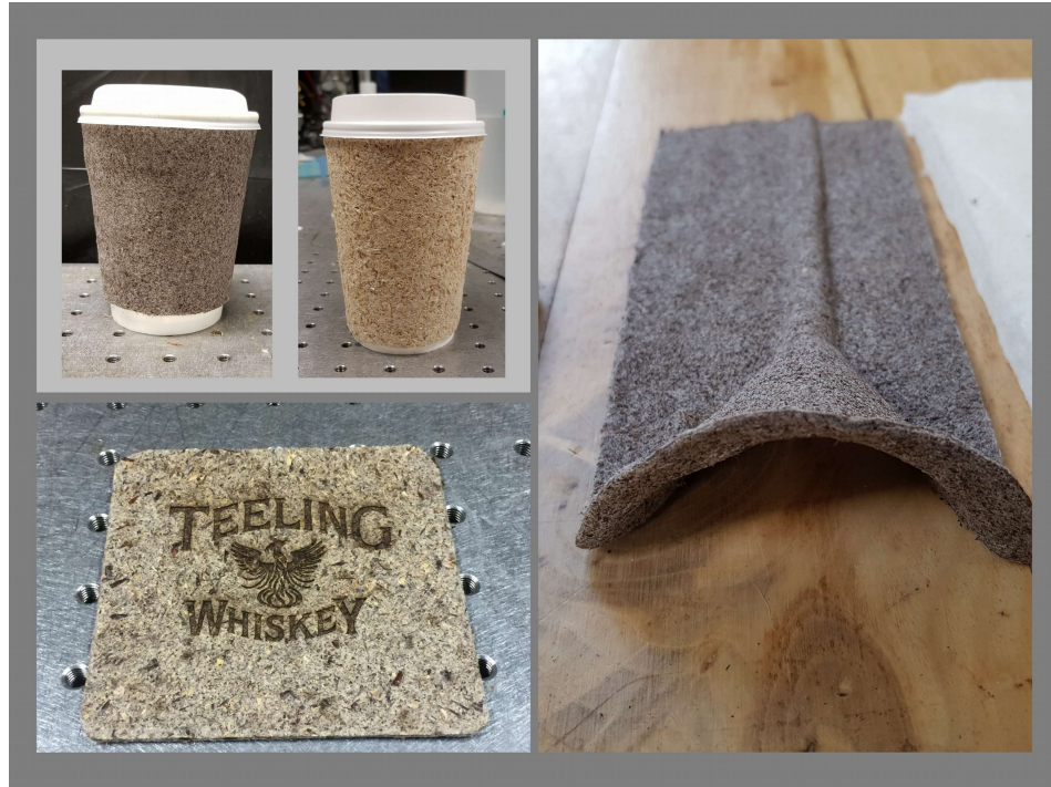
Fig 1.2: A selection of sheet-like materials made using recycled and recyclable fibres by way of the foam-forming technique. The top left picture shows insulating coffee cup wraps, designed to keep the hand cool when holding a hot beverage. The wrap on the left was made with peat fibres, while the one on the right was made with brewers spent grain. The bottom left picture shows a beer mat (drinks coaster) prototype also made of brewers spent grain. On the right is a moulded funnel, designed to show how other structures can be made from foam-formed fibrous sheets. All the materials in the above picture were made as part of this PhD project in our laboratory in Trinity College, Dublin.
