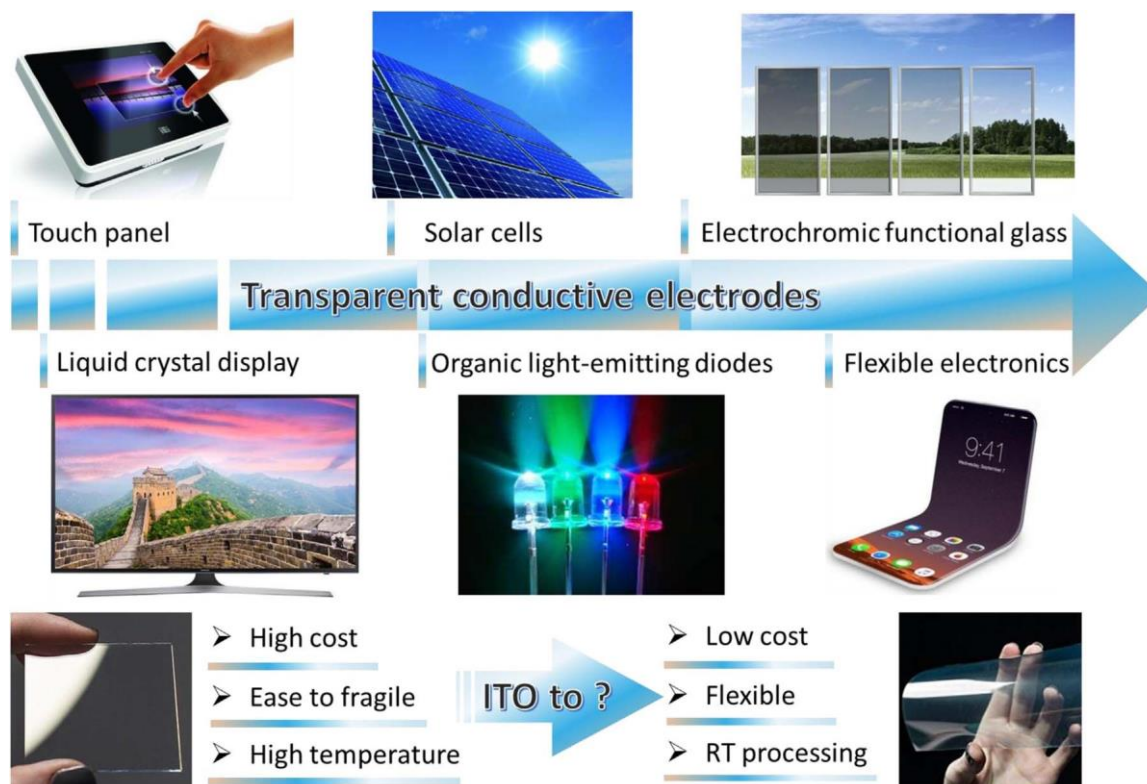
Fig. 1. Applications of transparent conductive electrodes. Also included are the current challenges of ITO and expected features in the ITO substitutes. Images are from the internet.
