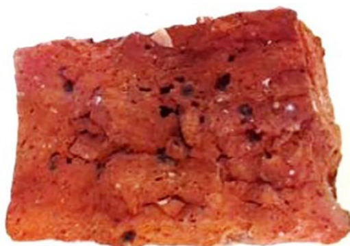
Figure 12 Specimen B12, represents the typical appearance of the high-temperature bricks. Photograph by Sara Pavia.
