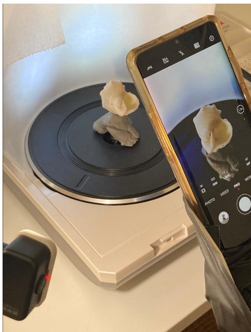
Image 10: Photography with a smart phone. The turntable is moved incrementally after each shot.
