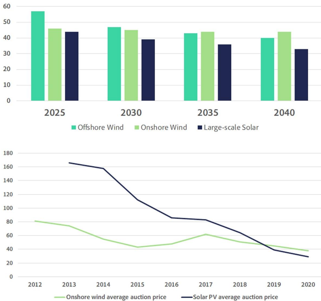
Figure 4.9 Auction prices for global onshore wind and solar PV in GBP per MWh (data source: IEA,, 2019)
