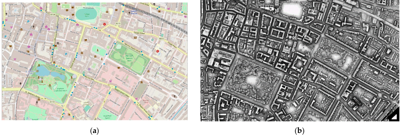
Figure 9. (a) The figure shows an OpenStreetMap image of the Dublin test area (© OpenStreetMap contributors) and (b) shows the right image shows the sky visibility at each point as modelled by the terrain shading algorithm in terms of no visibility (0 or black) to complete visibility of the upper hemisphere (1 or white). For the area shown here the median value of the upward hemisphere visible is 64%.
