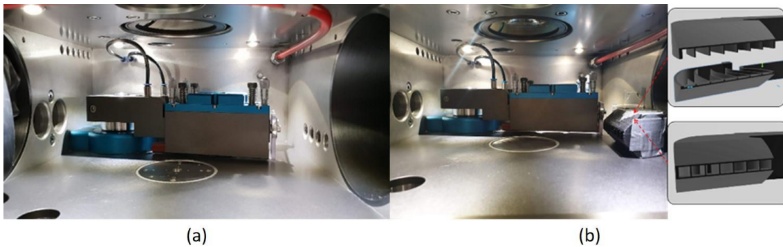
Figure 4.4: (a) Realizer nozzle configuration utilising four input holes on the right-hand side of the chamber and (b) the FDM printed nozzle inside the Realizer chamber
