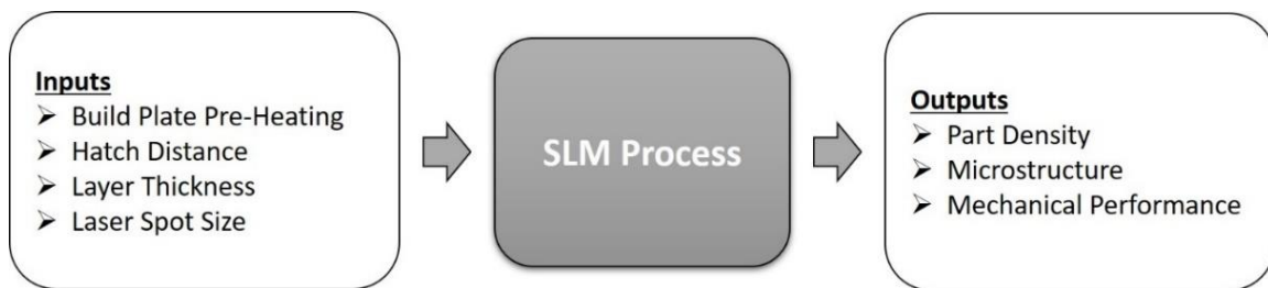
Figure 5.1: Flow diagram showing DOE used to explore as-built Ti64
