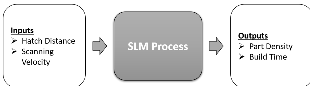
Figure 4.12: Flow diagram showing DOE process including build time
