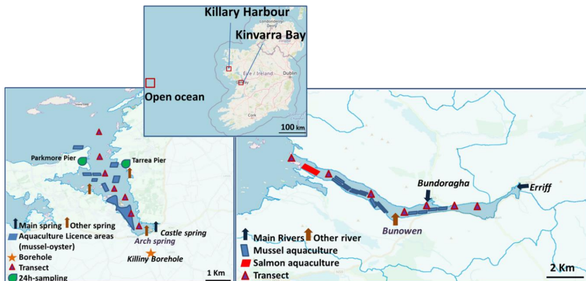
Figure 4-1: Kinvarra Bay and Killary Harbour bay sub-catchment areas from http://www.gis.epa.ie water framework directive units maps, together with major springs and rivers represented following Environmental Protection Agency reports (EPA 2011; Mara and Connolly 2016) are shown. Surface water sampling stations are marked with triangles. The areas where 24h fixed-point surveys were carried out in Kinvarra are also shown. The data collected in these two locations were used to build the tidal prism and to estimate the freshwater discharge. Aquaculture sites data were obtained from the Ireland's Marine Atlas at http://atlas.marine.ie/ on the 03/04/2020. The location of the open ocean data obtained from the Marine Institute (Galway) is represented in the central map.
