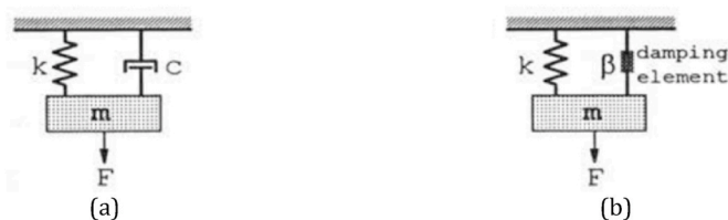
Fig. 10. (a) Kelvin-Voigt viscous damping model with inertia and (b) Complex Stiffness (CS) model (after [65]).
