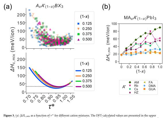
Figure 3. (a)  $\Delta H_{c,mix}$  as a function of  $\tau^*$  for different cation mixtures. The DFT-calculated values are presented in the upper panel, while the corresponding best fits are in the lower one. The colors encode the different cation concentrations investigated. (b)  $\Delta H_{c,mix}$  for MA<sub>x</sub>A'<sub>1-x</sub>PbI<sub>3</sub> and different A' cations (see legend) as a function of (1 - x).
