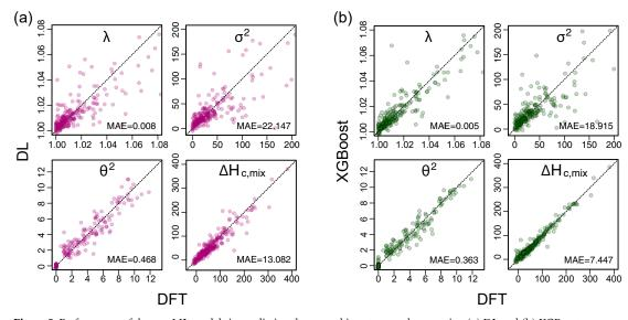
**Figure 5.** Performance of the two ML models in predicting the perovskites structural properties. (a) DL and (b) XGBoost predictions against the DFT data for  $\lambda$ ,  $\sigma^2$ ,  $\theta^2$  and  $\Delta H_{c,mix}$  (meV ion<sup>-1</sup>).
