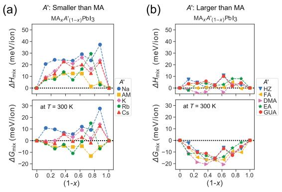
**Figure 4.** In panel (a) and (b) we plot the enthalpy of mixing,  $\Delta H_{mix}$  and the corresponding free energy at 300 K,  $\Delta G_{mix} = \Delta H_{mix} - T\Delta S$ , for MA<sub>x</sub>A'<sub>1-x</sub>PbI<sub>3</sub> perovskites. Panel (a) is for A' cations with ionic radius smaller than that of MA, while panel (b) is for those with a larger one. In evaluating the free energy  $\Delta S$  is the mixing entropy contribution, which reads  $\Delta S = k_B [x \ln(x) + (1-x) \ln(1-x)]$ .
