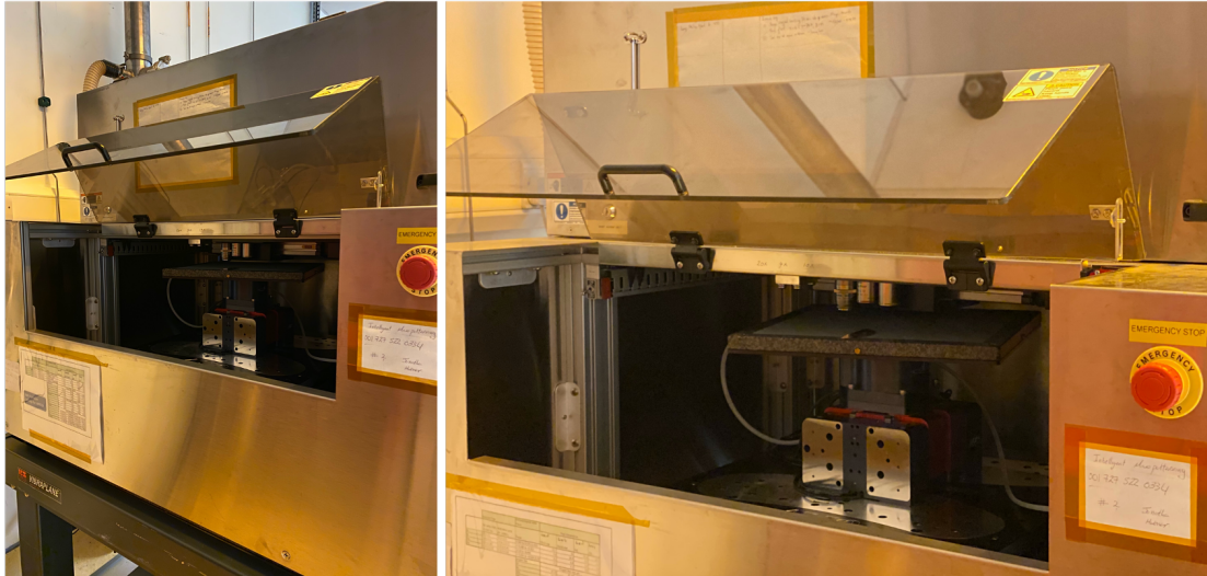
Figure 3.5: Photos of IMP tool used for maskless UV lithography.
