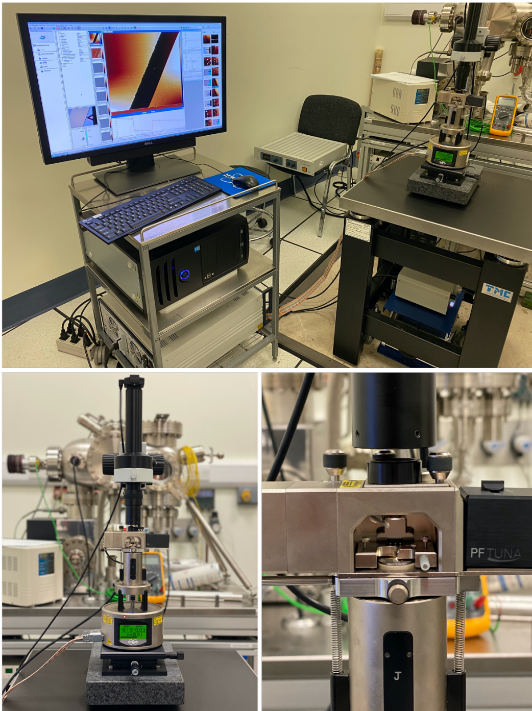
Figure 3.6: Photos of the Bruker Multimode 8 AFM, showing several components and aspects of the system.
