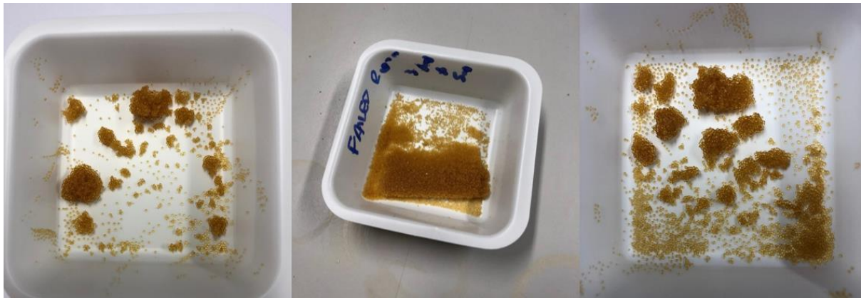
Figure 17. Images of failed Wurster coating runs using “blank” beads (IR120) and dibutyl sebacate (DBS) and triacetin (TCT) as plasticisers.
