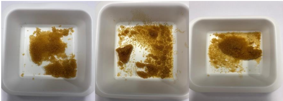
Figure 6. Images of unsuccessful Wurster coating runs (using “blank” IR120 beads) produced using Kollicoat® SR 30 D and Eudragit® NM 30 D.
