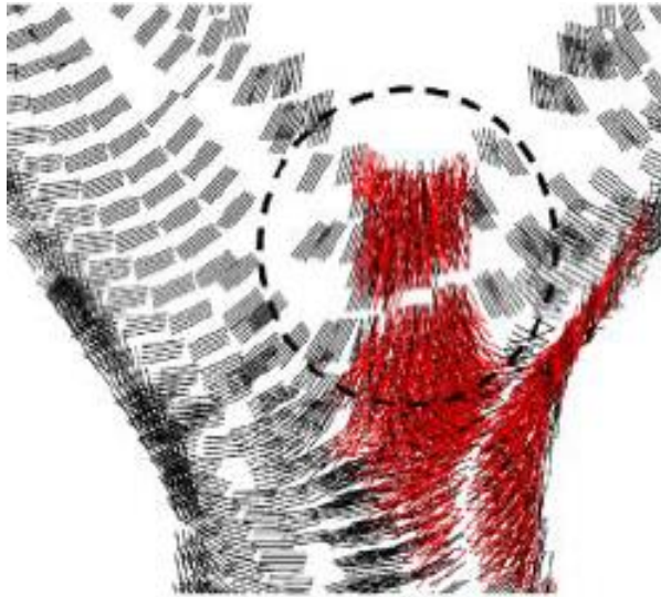
Figure 2.34 Principal stress segments (black) and collagen fibre orientation (red) at the carotid bifurcation. High alignment observed at the bifurcation apex [132]
