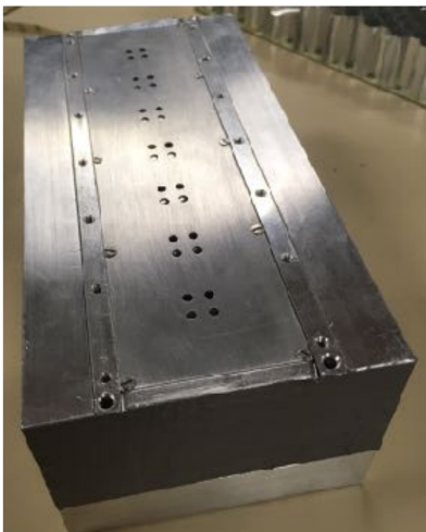
Figure B.7: Multilayered plates denoted as SET A in holder manufactured for test campaign with screws used to tighten the plates and spacers together.
