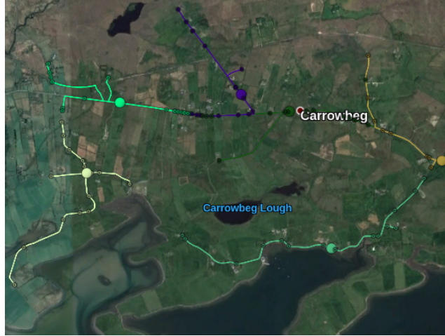
Figure 6.3: Sample outcome of fixed-size single-stage clustering, a number of 16-size clusters assembling separate end-users groups. A 16-size cluster denotes a drop section equipped with 1x16 power optical splitter. Every round coloured sphere indicates a cluster centre and the place where drop cables can be branched off from a splitter.
