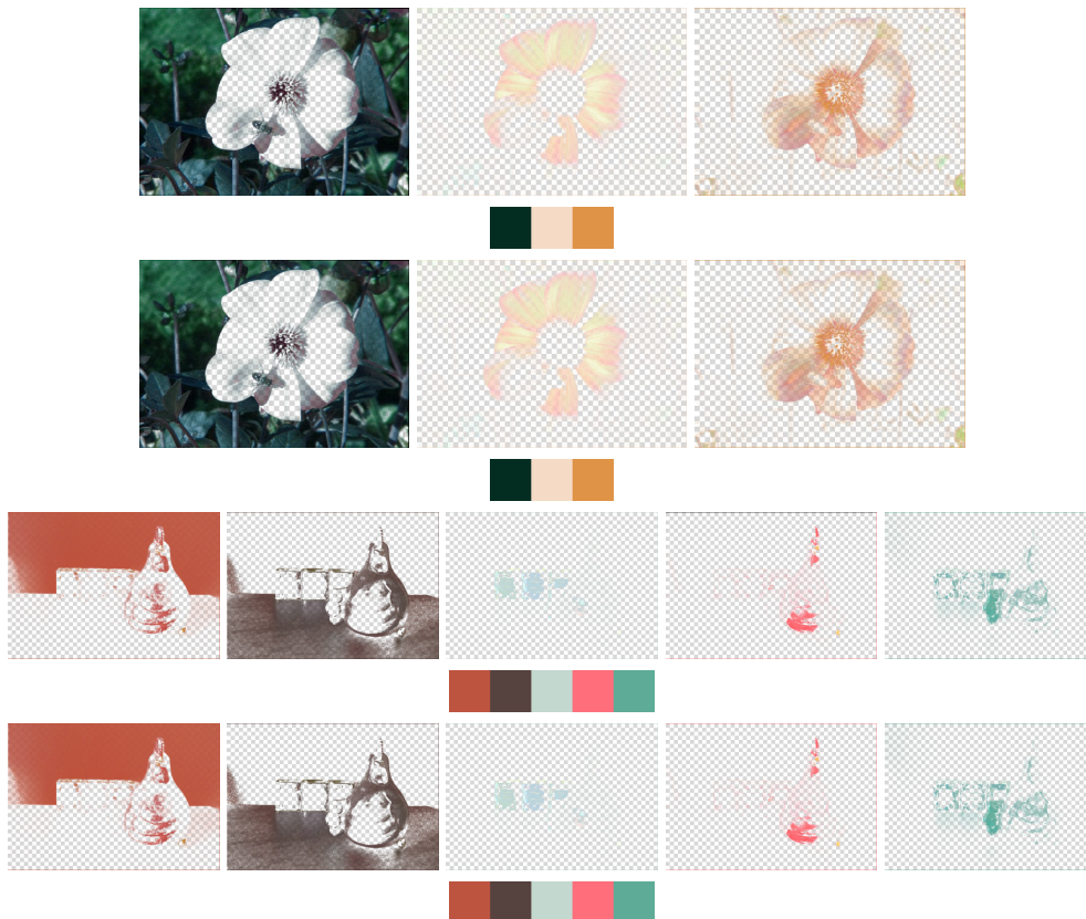
Figure 4.2: Results of our global approach to perform soft colour segmentation on the same consecutive views as in Figure 4.1. Compared to the naive approach here the number of layers is equal, and the colour distribution within layers is more consistent.
