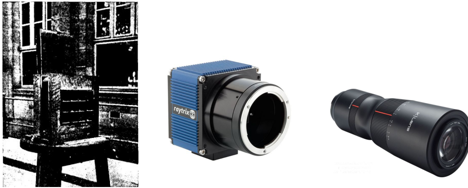
Figure 2.7: Various plenoptic devices. From left to right: Lippmann's integral photography device, showing here the front with its twelve lenses [46], Raytrix R11 3D light field camera [47], (h) K|Lens light field lens [48].
